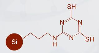
Loading: 0.83 mmol/g Surface Area: 525 m²/g Average Pore Size: 60Å Pore Volume: 0.79 cm³/g **Metals Targeted**
